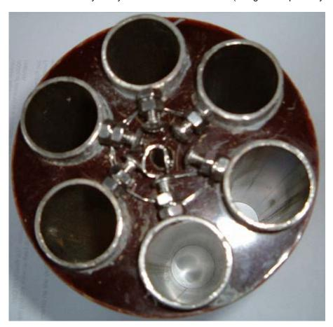
The electrical connections to the pipes are via stainless steel wire running between stainless steel bolts tapped into the pipes and stainless steel bolts running through the base of the unit:
